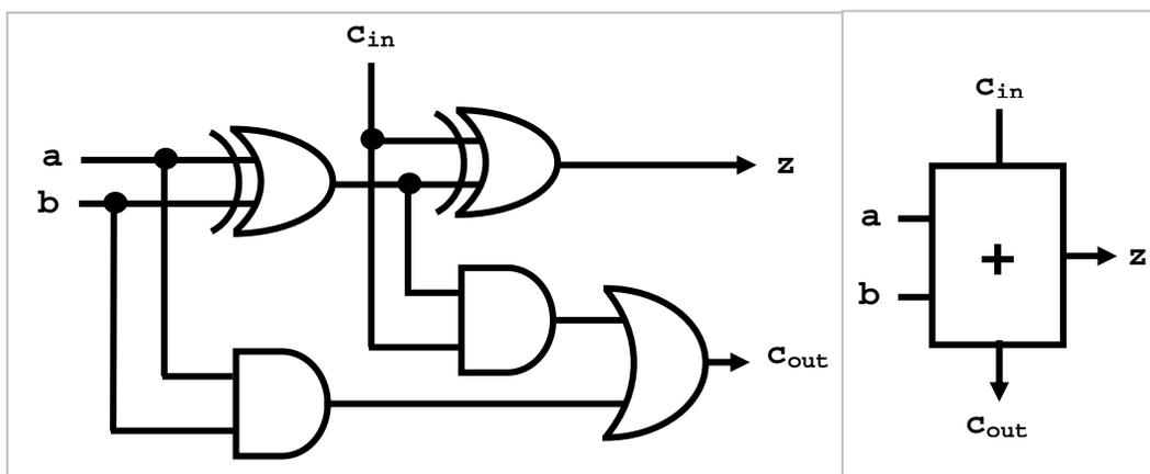
We now like to use abstraction to encapsulate this functionality. To that end, we repackage the adder as a component named **yAdder1** and having the block diagram shown in the right part of the figure (it operates on 1-bit wires and thus the **1** suffix).
