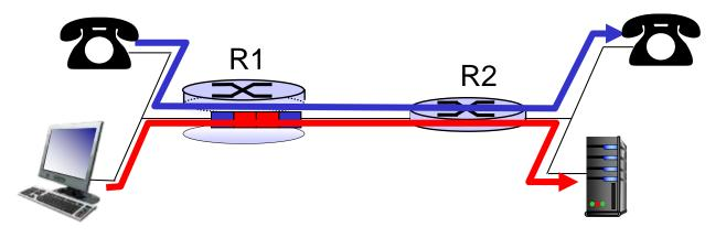
Principle I packet marking needed for router to distinguish between different classes; and new router policy to treat packets accordingly
