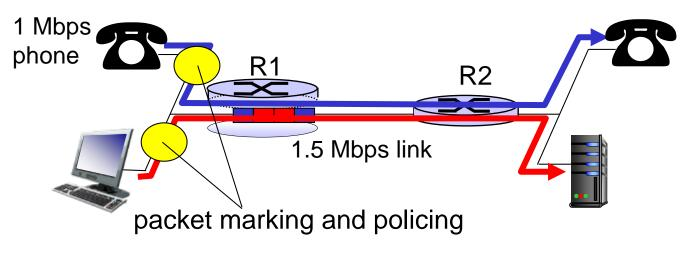
Principle 2 provide protection (isolation) for one class from others
