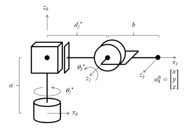
The prismatic joint of the robot has length  $5 \le d_2^* \le 10$ . The range of joint 1 is  $0^\circ \le \theta_1^* < 360^\circ$  and the range of joint 3 is  $-170^\circ \le \theta_3^* \le 170^\circ$  The exact values of a and b are not important, but assume that a > b and b < 5.
