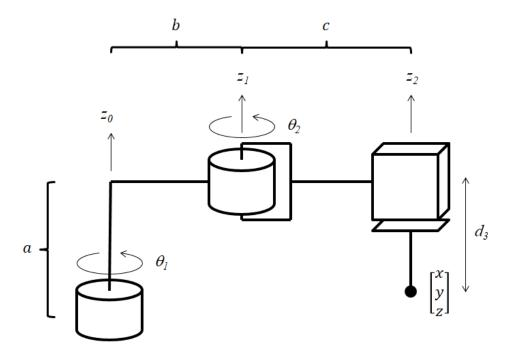
The robot is shown in a position where all of the joint angles are zero degrees and  $d_3$  is some positive value. For the purposes of this question, assume that there are no limits on the joint parameters.
