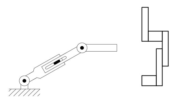
(b) Given the end effector position (say at the end of link 4), solve for the inverse kinematics of the robot.
