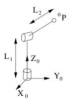
(d) Consider the robotic arm shown below made up of a prismatic joint (moving vertically) and a revolute joint (positive rotation counter-clockwise in the page). Derive the matrix  $T_3^0$ . Assume that the frames shown indicate the X and Y axes of the frames. Do not use the Denavit-Hartenberg convention to obtain a solution; the manipulator is simple enough that you should be able to derive a solution using basic linear algebra.
