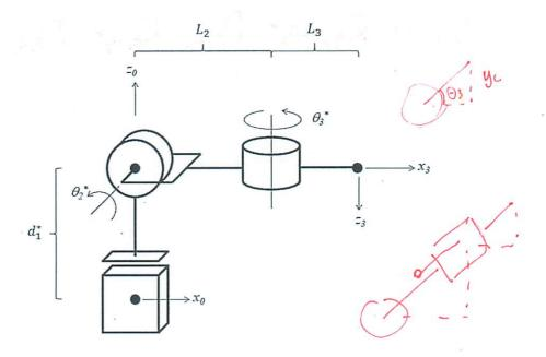
The robot is shown in a position where all of the joint angles are zero degrees.
