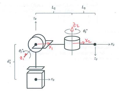
The robot is shown in a position where all of the joint angles are zero degrees. For the purposes of this question, assume that there are no limits on the joint angles and that  $d_1^* > 0$ .
