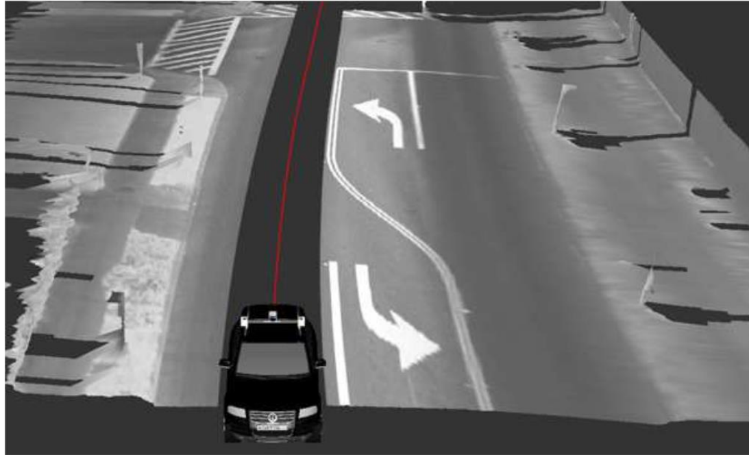
Figure 9: The side lasers provide intensity information that is matched probabilistically with the RNDF for precision localization.
