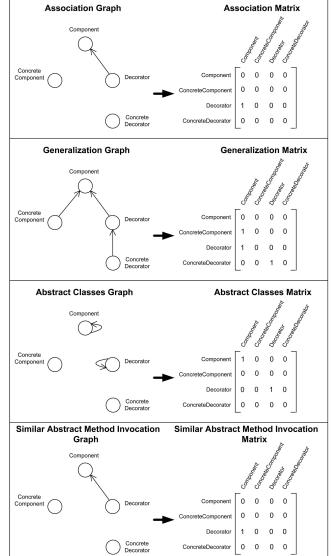
Fig. 2. Representation of pattern structure as graphs and matrices.
