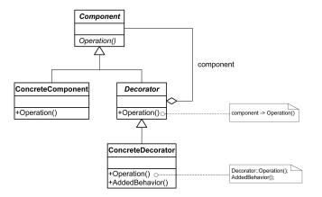
Fig. 1. Structure of decorator design pattern.
