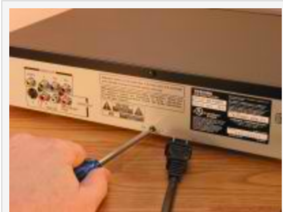
Remove screws from the rear of the case to remove the top and access internal components.
