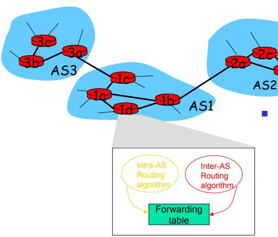
Forwarding table is configured by both intraand inter-AS routing algorithm
