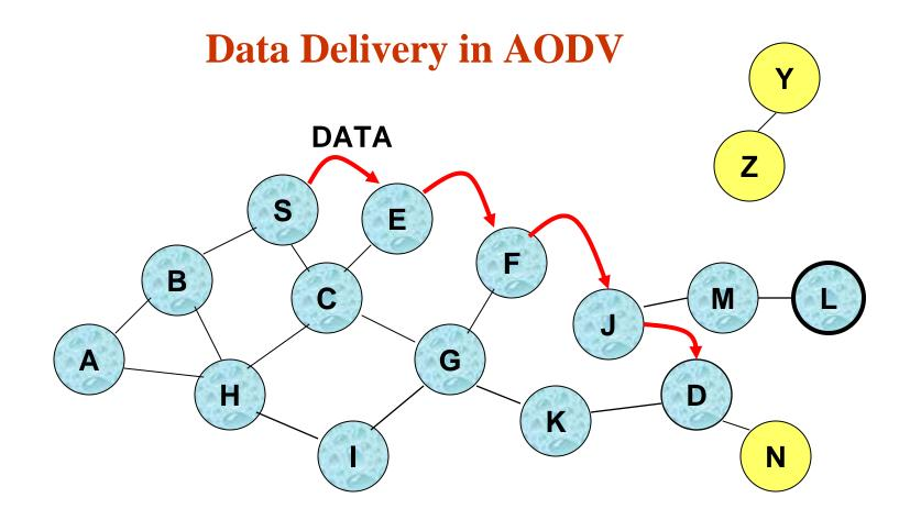
Routing table entries used to forward data packet.
