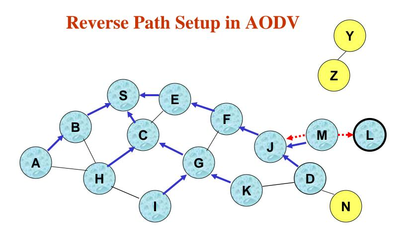
• Node D does not forward RREQ, because node D is the intended target of the RREQ
