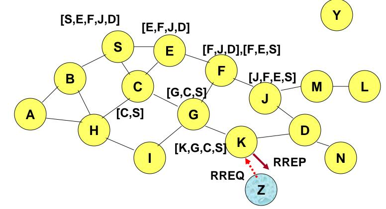
Assume that there is no link between D and Z. Route Reply (RREP) from node K limits flooding of RREQ. In general, the reduction may be less dramatic.
