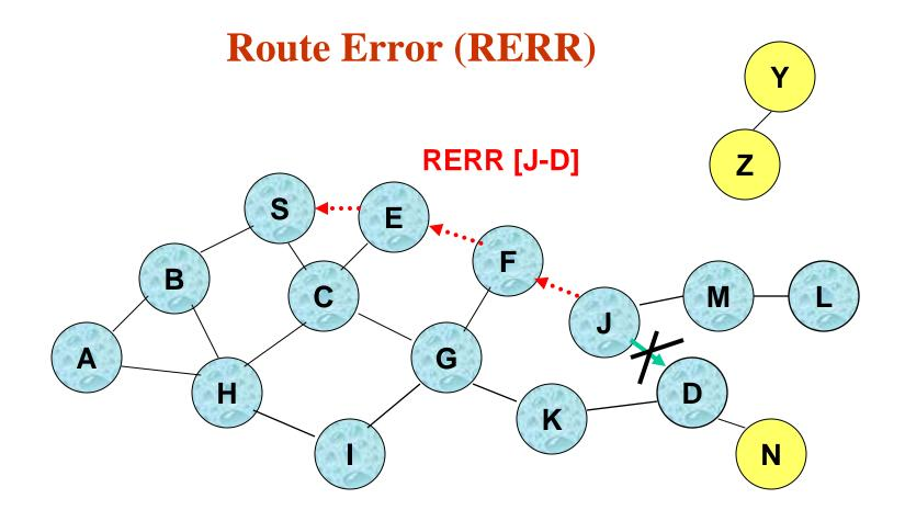
J sends a route error to S along route J-F-E-S when its attempt to forward the data packet S (with route SEFJD) on J-D fails
