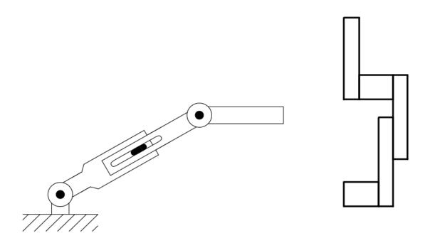
(b) Given the end effector position (say at the end of link 4), solve for the inverse kinematics of the robot.
