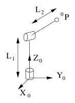
(d) Consider the robotic arm shown below made up of a prismatic joint (moving vertically) and a revolute joint (positive rotation counter-clockwise in the page). Derive the matrix  $T_3^0$ . Assume that the frames shown indicate the X and Y axes of the frames. Do not use the Denavit-Hartenberg convention to obtain a solution; the manipulator is simple enough that you should be able to derive a solution using basic linear algebra.
