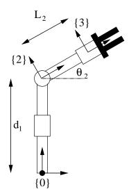
6. (a) Consider the figure shown below of a PP robot (left: view of the side of the robot, right: view of the front of the robot). Derive the forward kinematics of the robot using the DH-convention; choose your own variables for the missing dimensions.
