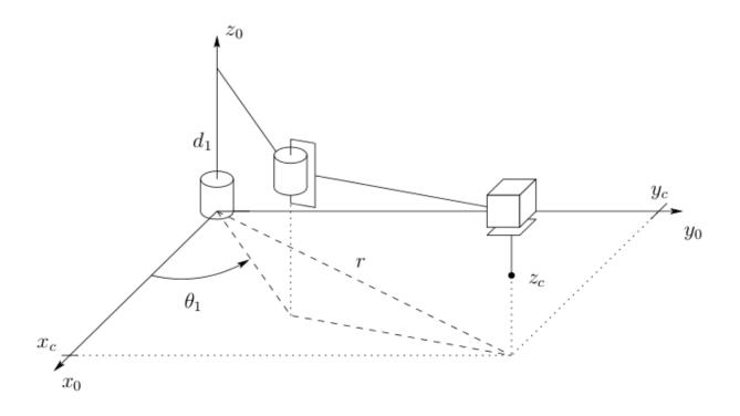
(b) Given the wrist center location  $[x_c y_c z_c]^T$ , solve for the inverse kinematics of the robot.
