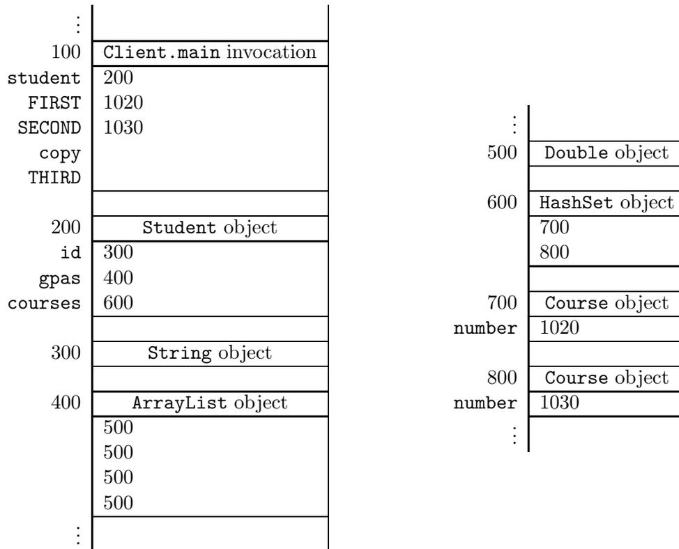
Since the class `Double` implements the pattern “one instance per state”, the above memory diagram contains only a single `Double` object.
