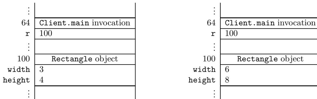
The memory diagram above assumes that the `Rectangle` object resides in a memory block that starts at address 100. The diagram shows that the value of `r` was 100 before the invocation and remained 100 after it, as expected. The object itself was mutated as evidenced by the doubling of its sides. The fact that the object was changed does not contradict the pass-by-value mechanism because the object itself is not an argument; its reference is.<sup>5</sup>
