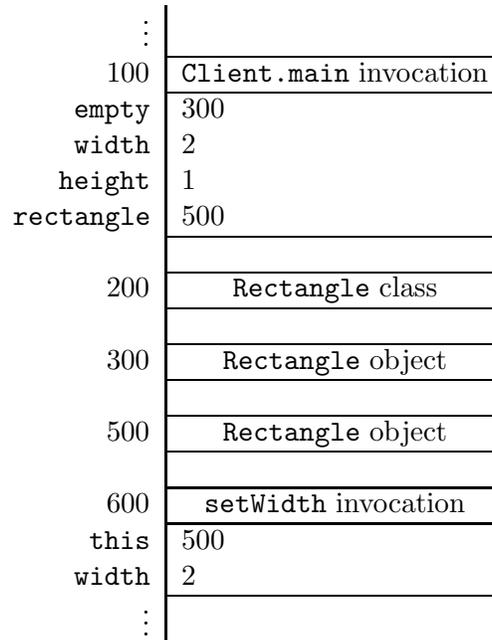
The diagram shows an invocation block for the `main` method of the `Client` class, a class block for the `Rectangle` class, two object blocks for the two created `Rectangle` instances, and an invocation block for the `setWidth` method. Recall that, in the client's concern, an invocation block contains one entry for each argument passed to the method. For the implementer, this is true only if the
