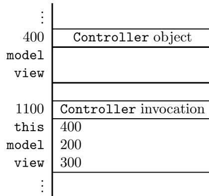
Once we reach the end of the constructor of the `Controller` class, the `Controller` object can be depicted as follows.
