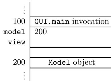
When executing line 2 of the GUI app, a memory block for the `View` object is allocated and the constructor of the `View` class is invoked.
