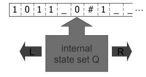
At every step, the head of the TM M reads a letter x<sub>i</sub> from the one-way infinite tape.
