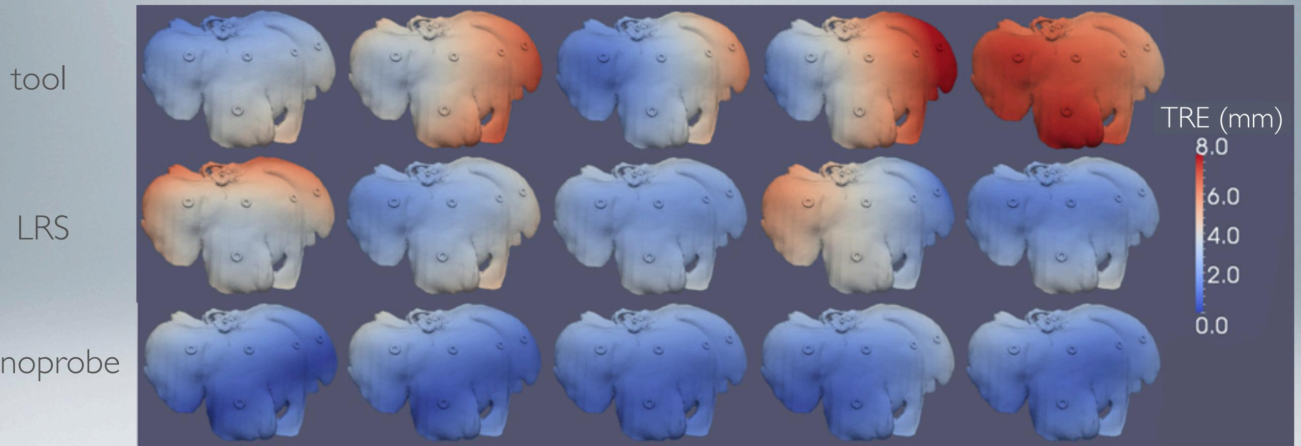
TRE computed using data from three acquisition methods for five trials. TRE increases from blue to white to red.
