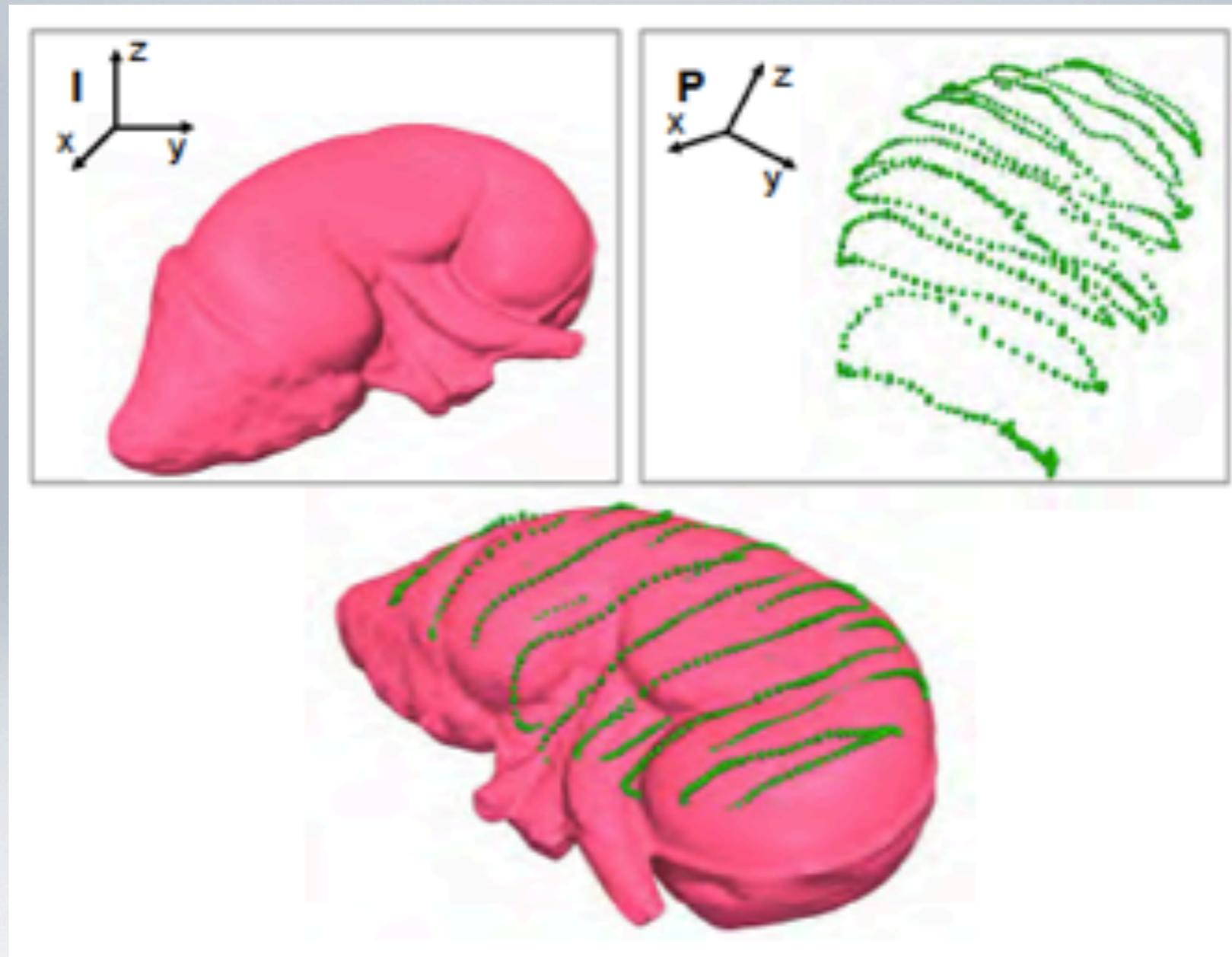
Surface model of anthropomorphic kidney phantom and the conoscopic point data after surface registration.
