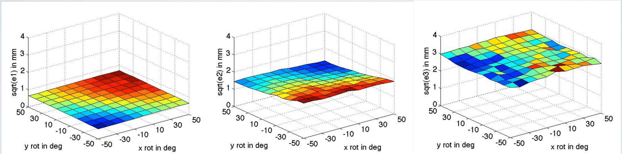
A sample covariance in tip position ( $x, y, z$ ) measured by our model when registration and calibration covariance are factored in.
