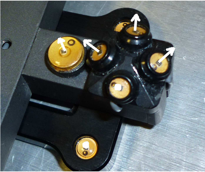
Fig. 5. An example of surface normal vectors on the cross rigid body
