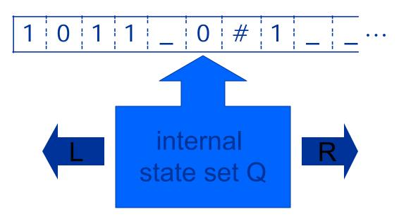
At every step, the head of the TM M reads a letter x<sub>i</sub> from the one-way infinite tape.
