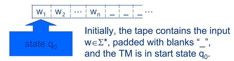
During the computation, the head moves left and right (but not beyond the leftmost point), the internal state of the machine changes, and the content of the tape is rewritten.
