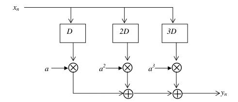
A more efficient implementation will use one delay line of length 3D and tap out the signal after D and 2D. In this case we used 3D delay elements (buffers in your program) instead of 1+2+3=6D delay elements
