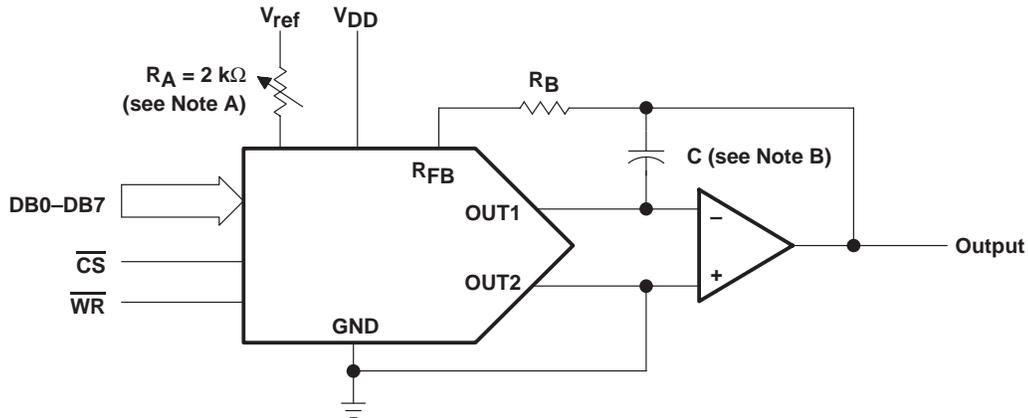
NOTES: A.  $R_A$  and  $R_B$  used only if gain adjustment is required.
