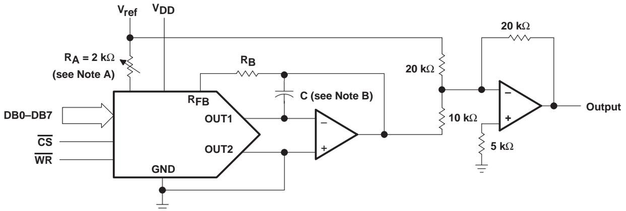
NOTES: A.  $R_A$  and  $R_B$  used only if gain adjustment is required.
