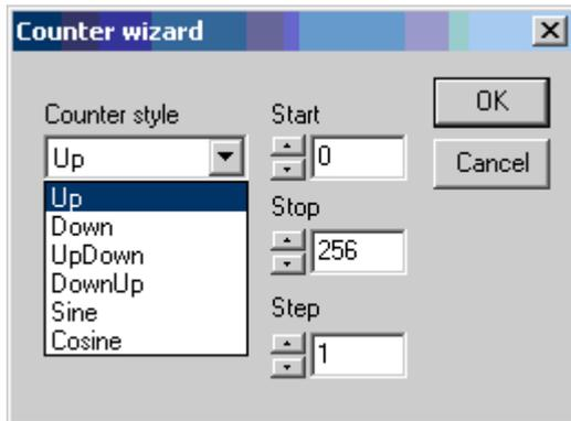
Use this window to generate a counter within the Pattern Generator data. The counter will be created within the currently [selected region](#).
