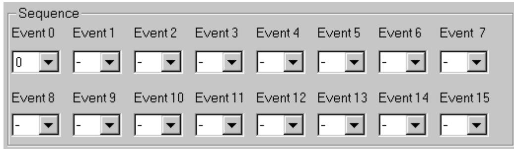
Use the list boxes to select which condition from the library of trigger patterns you want in each trigger level. Any level set to "-" will be skipped.
