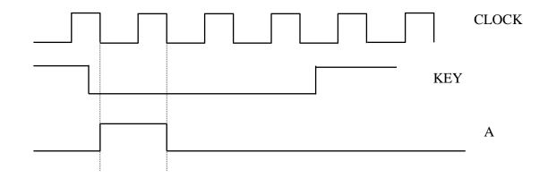
As you can see from the above diagram, when one of the keys is pushed (to ground), one pulse is generated at the trailing edge of the clock for a one clock cycle. For every input, you have to use a one-shot with the output of the one-shot going to the finite state machine.
