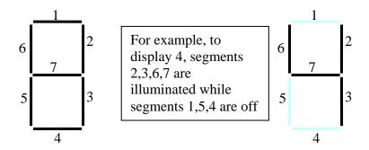
The seven segment display consists of 7 LEDs as shown in the above figure, the different LEDs are switched on and off to represent a certain number, so for example to represent the number 4, LEDs number 2,3,6 and 7 are ON the rest are off.
