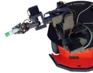
Figure 1. The Pioneer Arm on a 3-DX
