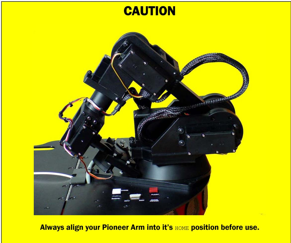
1. Put the Pioneer Arm into its HOME position: The tip of the Arm's V-shaped mounting base should point towards the rear of the robot, and the arm should be folded towards the back of its base.
