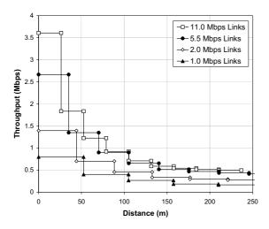
Figure 6: Throughput Loss Along a Path
