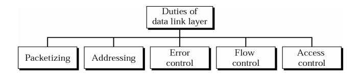
Why Error – data sent from one computer to another should be transferred reliably – unfortunately, the physical link cannot guarantee that all bits, in each frame, will be transferred without errors
