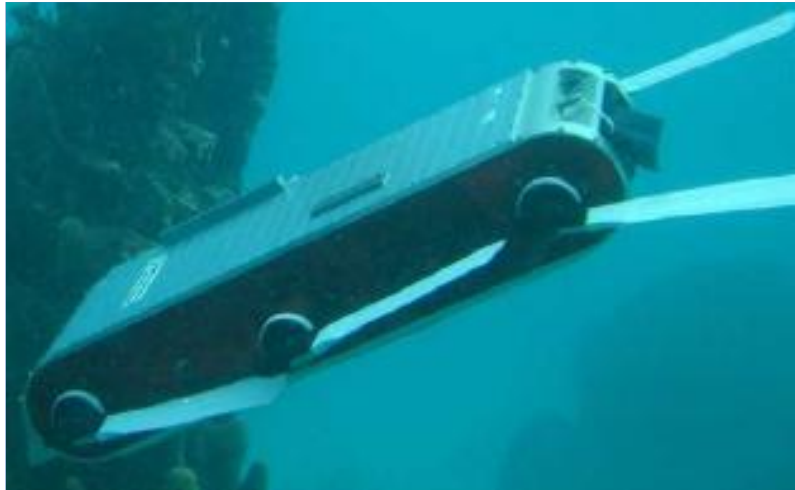
The AQUA submersible robot [3].
