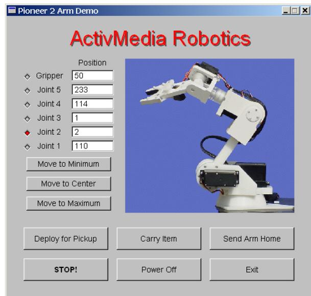
Figure 5. The `P2ArmDemo` lets you operate the Pioneer Arm quickly and easily.
