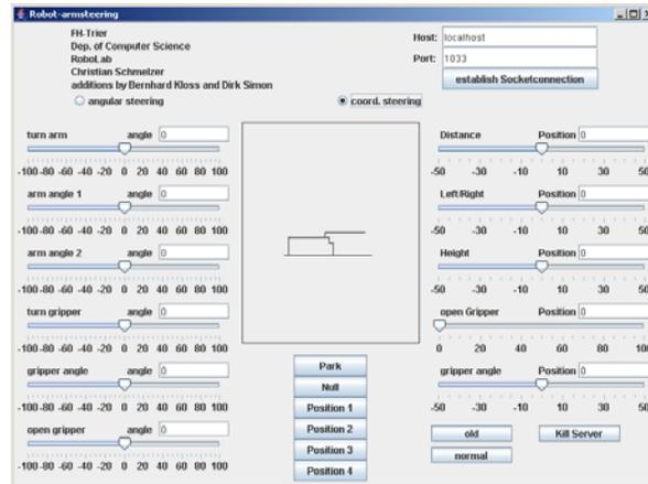
Figure 6. Connect `ArmApplet.jar` GUI to `ArmServer` to steer the arm with AKIN-based kinematics.
