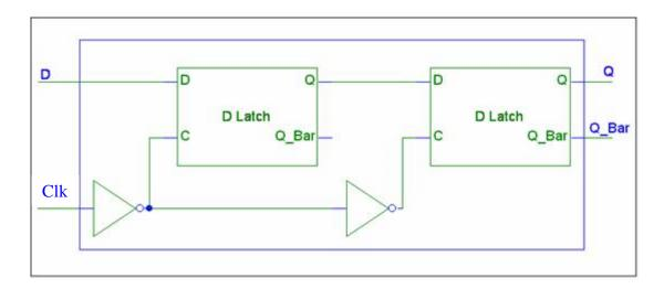
Using the previously designed module, implement the above circuit. Use the appropriate waveforms to test it.
