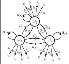
S =  $\omega_1$ ,  $\omega_3$ ,  $\omega_2$ ,  $\omega_2$ ,  $\omega_1$ ,  $\omega_3$  (hidden)  $\downarrow \qquad \downarrow \qquad \downarrow \qquad \downarrow \qquad \downarrow$ O = v4, v1, v1, v4, v2, v3 (observed)
