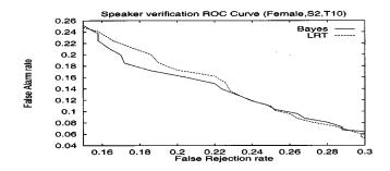
Fig. 5. Comparison of speaker verification ROC curves for female speakers under training condition s2 and test condition T10. Dotted-line: likelihood ratio test (LRT), solid-line: Bayesian approach (Bayes).
