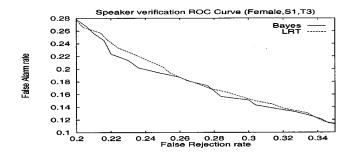
Fig. 3. Comparison of speaker verification ROC curves for female speakers under training condition s1 and test condition T3. Dotted-line: likelihood ratio test (LRT), solid-line: Bayesian approach (Bayes).
