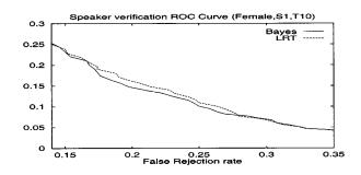
Fig. 2. Comparison of speaker verification ROC curves for female speakers under training condition **s1** and test condition **T10**. Dotted-line: likelihood ratio test (LRT), solid-line: Bayesian approach (Bayes).
