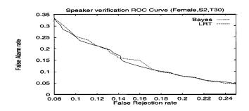
Fig. 4. Comparison of speaker verification ROC curves for female speakers under training condition **s2** and test condition **T30**. Dotted-line: likelihood ratio test (LRT), solid-line: Bayesian approach (Bayes).
