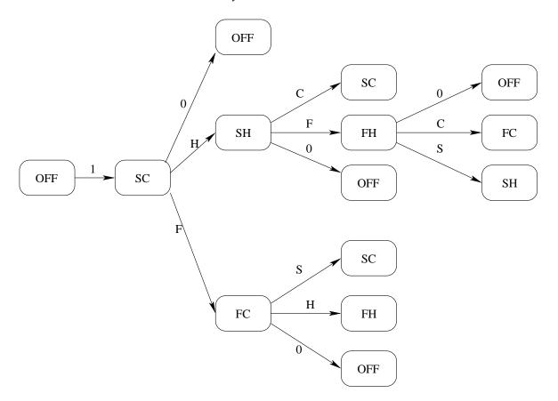
Each one of the paths from the alpha state to a leaf node in the tree is one test case. The sneak path test suite covers all possibilities not mentioned in the state transition diagram [8 marks]
