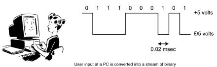
digits (1s and 0s). In this graph of a typical digital signal, binary one is represented by Đ5 volts and binary zero is represented by +5 volts. The signal for each bit has a duration of 0.02 msec, giving a data rate of 50,000 bits per second (50 kbps).
