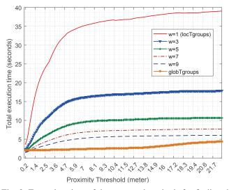
Fig. 8: Execution time of the proposed methods for finding the pedestrian groups in the **entire** video ( $\approx 1$  hour) for varying proximity threshold  $\tau$ .
