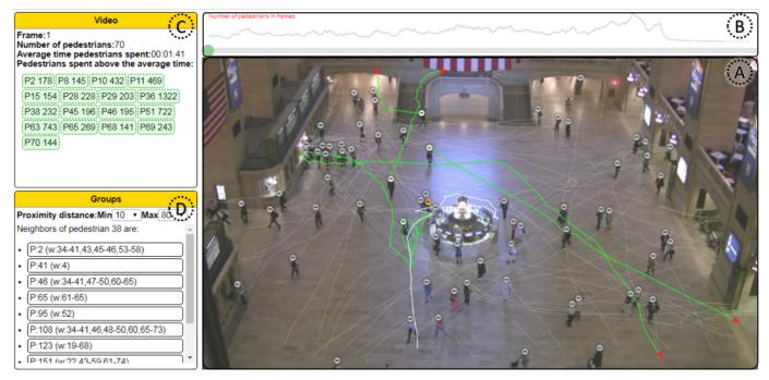
Fig. 9: Snapshot of the tool that allows for an interactive exploration of pedestrian group dynamics.
