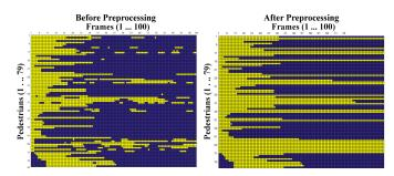
Fig. 4: Left and right maps show the trajectories before and after filling the unreported stationary positions respectively. Yellow cell indicates the reported (x, y) coordinates of moving pedestrian and the blue cell indicates the unreported position of stationary pedestrian.
