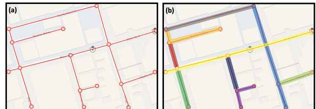
Figure 1: (a) Graph representation of a small area in Toronto 1 ; (b) Example of various-length edge-disjoint pathlets in (a).
