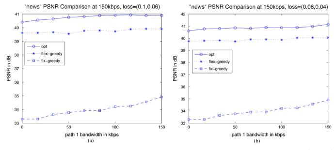
Fig. 9. Streaming performance for news in PSNR for varying path-1 bandwidth for fixed total bandwidth = 150 kbps. (a) loss rate = (0.10, 0.06). (b) loss rate = (0.08, 0.04).
