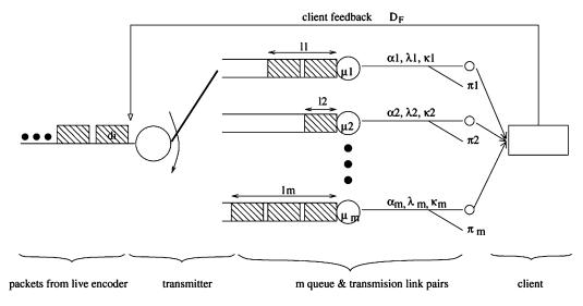
Fig. 8. Network simulator muns is used to simulate queuing, transmission, and losses of packets.
