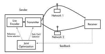
Fig. 1. Application scenario of interest involves live streaming with feedbacks over multiple network interfaces. The sender is responsible for jointly selecting the reference frames and associated QoS levels on multiple transmission paths. An effective scheme to realize such joint optimization is the focus of this paper.
