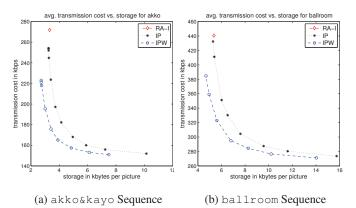
Fig. 4. Tradeoffs between Expected Transmission Rate and Storage per Picture for Various IMVS Schemes
