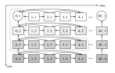
**Fig. 1**. A 4-view, 5-instant Example of Multiview Frame Structure using Inter-view Prediction for Key Frames in [1].
