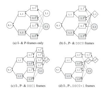
Fig. 3. IMVS structures for two views (two shades). I-, P- and DSC frames are denoted as circles, squares, and diamonds respectively.
