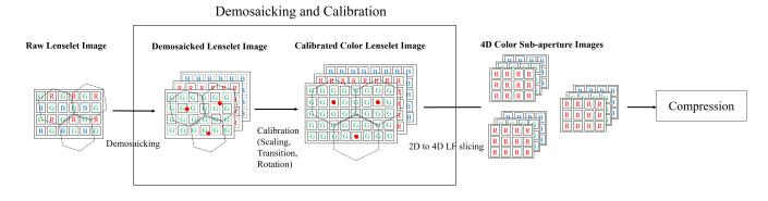
Fig. 1: Conventional coding scheme for light field image. The demosaicking and calibration processes are applied before compression.
