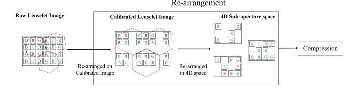
Fig. 2: Proposed LF coding scheme. The demosaicing and calibration, yielding high signal redundancy, are applied after compression.
