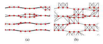
**Fig. 4**: A part of graph constructed for irregularly placed R components. In (a), the one using 4 nearest neighbor method is shown. In (b), each pixel is connected to 2 neighbors in horizontal and vertical orientations respectively
