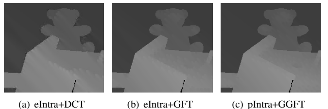
Fig. 4. The subjective quality comparison among different compression schemes. (a) ~ (c) Teddy at 0.10 bpp.
