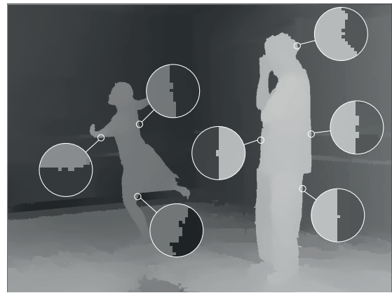
Fig. 2. Example of depth irregularities along boundaries, which make harder the prediction of the geometrical structure of the boundary.
