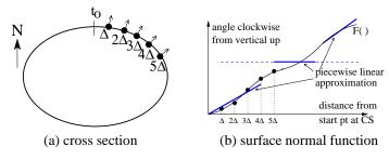
Fig. 2. Example of cross section and surface normal function.
