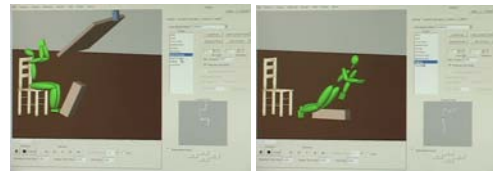
Figure 4: The user controls the 3D character interactively. The controllers are chosen at a timing indicated by the user, and can be simple pose based controls or complex, scripted controllers.
