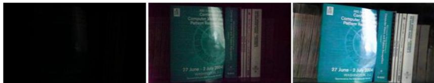
(a) Camera output with ISO 8,000 (b) Camera output with ISO 409,600 (c) Our result from the raw data of (a)
