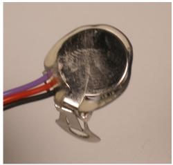
Allow the hot glue to ooze out around the ear clip. That will ensure good coverage. Take care not to let the hot glue cover around the ear clip hinge, as that could get in the way of it working. Trimming is easy with nail clippers (as above) or your trimming tool of choice. Don't trim the wires by mistake!!!
