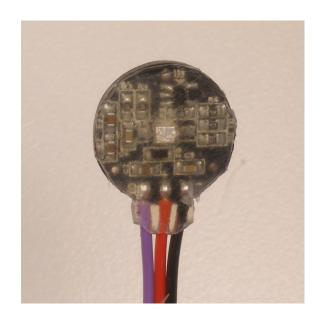
This is the basic Pulse Sensor Hot Glue Seal, It's also got the clear vinyl sticker on the front face. We're calling this 'Water Resistant', ready to be handled and passed around from fingers to earlobes or whatever. It is not advised to submerge or soak the Pulse Sensor with this basic seal.
