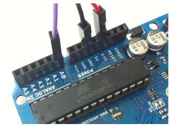
Then, run the processing sketch and see if you get a better wave shape. If you see a nice bright pulse waveform, then hooray! this is your fix! Notice, however that the pulse wave is in the lower portion of the pulse window. That's because of the difference in voltage between the power to the Pulse Sensor (3.3V) and the voltage reference to the Arduino (5V)
