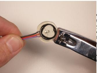
Once the hot glue has cooled (wait for it!) the blue tape will peel off very easily. Check your work to make sure that there are not exposed electrical connections!
