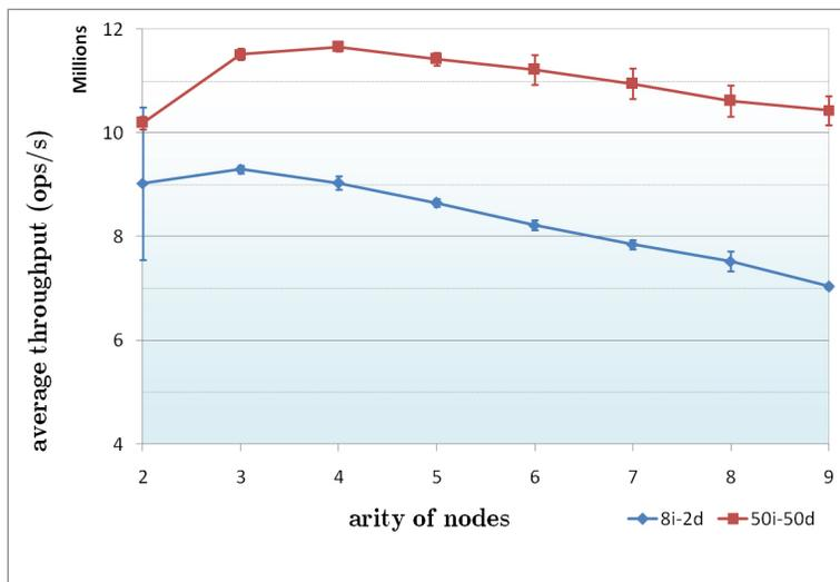
Figure 23: Comparison of the throughput of  $k$ -ary search trees with ratios 2i-8d and 50i-50i, and key range  $10^6$ , as  $k$  varies between 2 and 9.
