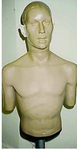
Figure 3.2: KEMAR Mannequin. The KEMAR (Knowles Electronic Mannequin for Acoustic Research) is often used to obtain HRTF measurements. Reprinted from [82].
