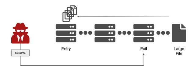
This process is repeated until the memory of the entry relay is used up
