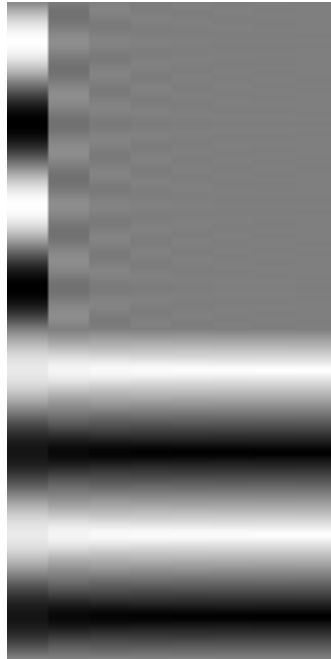
Fig. 2.4 The image on the left shows the a series of strips whose intensity approximates the sawtooth pattern. The first strip contains one component, so it is just a sine, the second two etc. The ridges become successively sharper. The image on the right shows the components.
