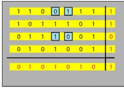
e. Four errors cannot be detected
