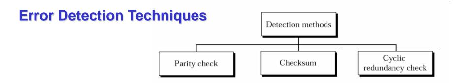
Single Parity Check – take k information bits and append a single check (Even Parity) bit so that <u>overall number of 1s is even !</u>
