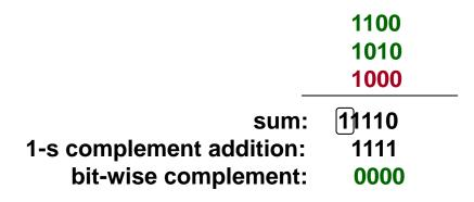
When the receiver adds the three blocks, it will get all 1s, which, after complementing, is all 0s and shows that there is no error.
