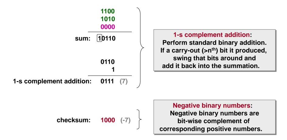
Suppose the receiver receives the bit sequence and the checksum with no error.
