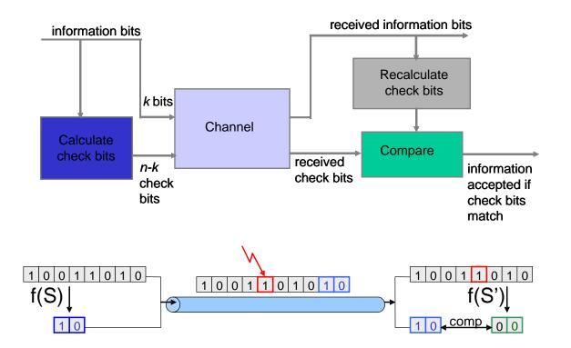
Modulo 2 arithmetic is performed digit by digit on binary numbers. Each digit is considered independently from its neighbours. Numbers are not carried or borrowed.
