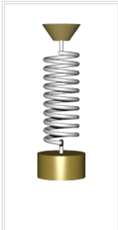
The oscillation of an undamped spring-mass system around the equilibrium is a sine wave
